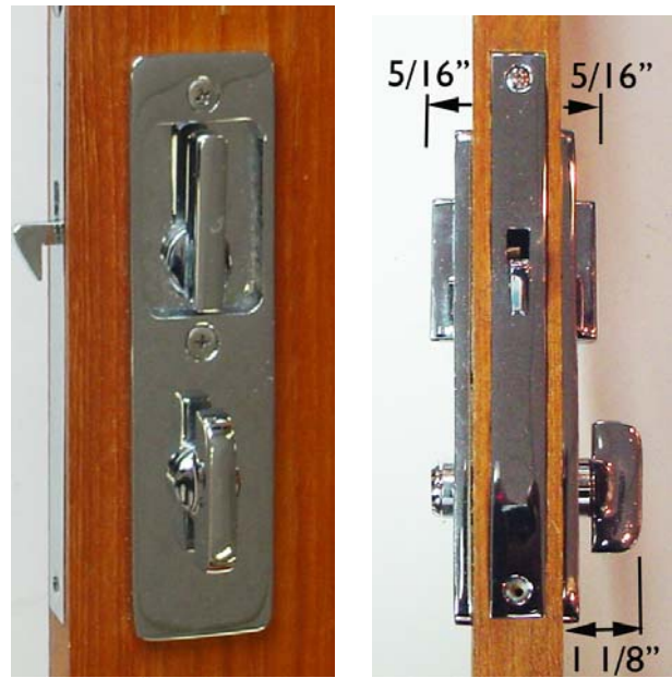
SET: #16.99W privacy with knob / indicator MINIMUM DOOR THICKNESS: 1" ;
